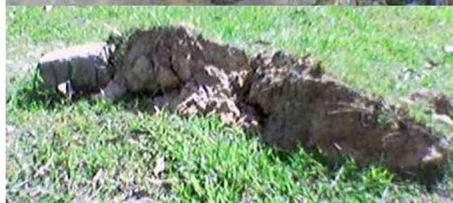
➤ exploded 132 kV joint after cable fault, 132 kV XLPE, explosion lifted soil above the faulty spot.
