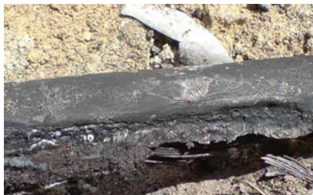
➤ vaporized core after cable fault, 132 kV XLPE
