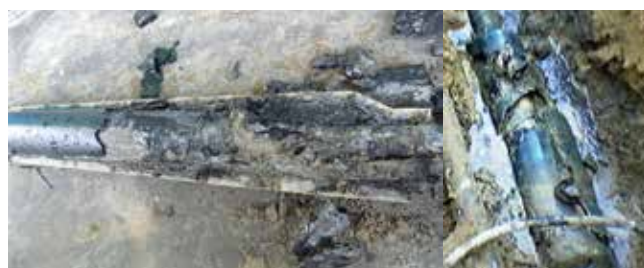
➤ vaporized core after cable fault, 132 kV XLPE
