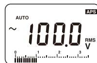
Measuring 100 V using the 300 V range
