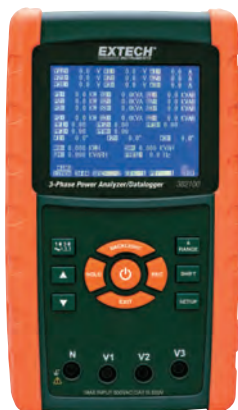
Model 382100 includes 1200A Clamp Probes
