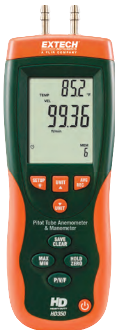
Includes pitot tube with two 33.5" (85cm) connection hoses
