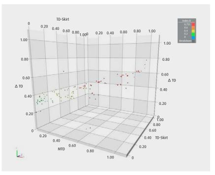
Figure 7: Representation of ageing index R (see legend) for all measured phases as a three-dimensional diagram. Each point represents the condition of a measured phase.
