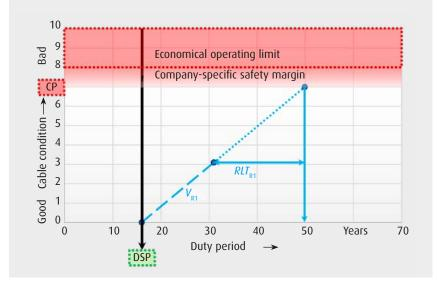
Figure 5: The statex software can use the tan  $\delta$  measured values to calculate the ageing index and estimate the remaining life time of the cable.
