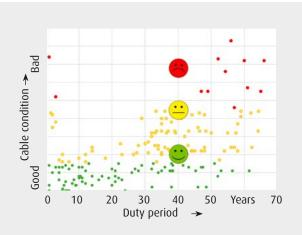
Figure 2: With condition-oriented network maintenance based on diagnostic measurements, old intact cables can continue to be used and newer cables that are in poor condition can be detected promptly and replaced. This minimises costs and increases the availability of the network.
