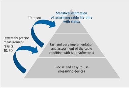
Figure 3: With the new statex software, the values from the dissipation factor measurement can be used to predict the remaining life time of medium-voltage cables.
