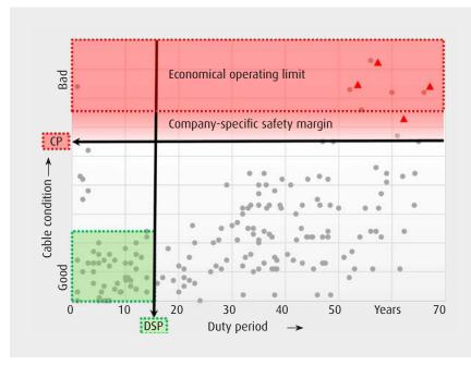
Figure 4: Typically, the ageing process for XLPE cables only begins after more than ten years when the antioxidants in the cable insulation have outgassed and water trees start to form.
