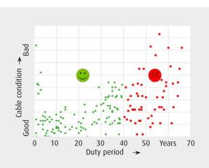
Figure 1: A strategy for replacing cables based on absolute age would mean that many cables that are still intact (as illustrated in the bottom right area of the diagram) would be replaced.
