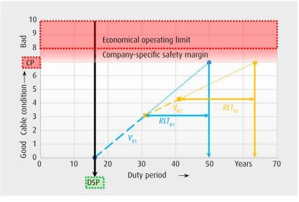
Figure 6: statex recalculates the remaining life time when repeat measurements are performed.
