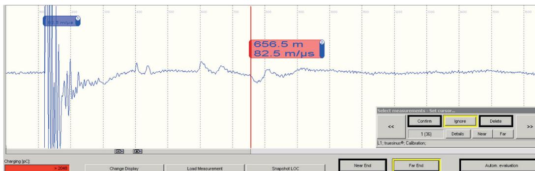
➤ Figure 78: TDR / calibration graph with identification of joint with water ingress at 656.5 m
