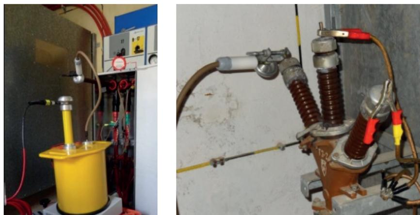
Figure 121: MWD diagnostics on aged cable system – PD TaD 62
