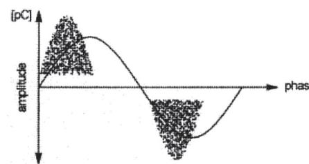
Figure 85: Inner partial discharge source, incomplete shrinking in heat shrink joint, PRPD pattern
