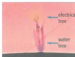
➤ Figure 27: Water tree with developing level of electrical tree, PD activity
