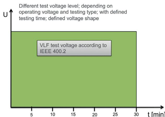
Figure 3: Simple VLF Test according to IEEE 400.2 [11]
