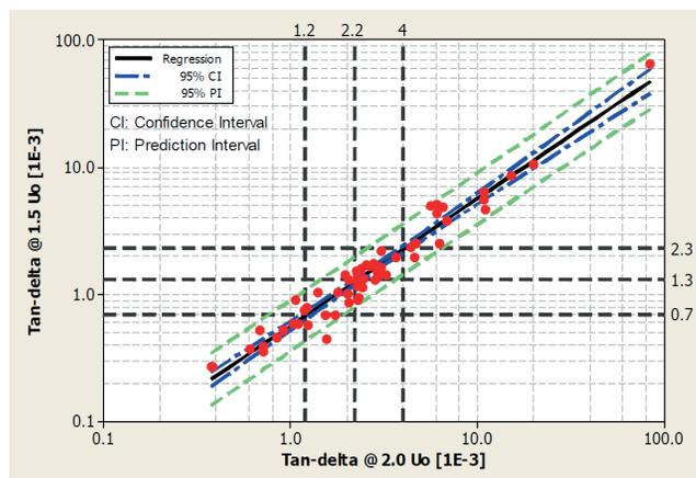
➤ Figure 33: Correlation between tan delta measurements from field testing at  $2.0 U_0$  and  $1.5 U_0$  for modified diagnostic criteria [18]
