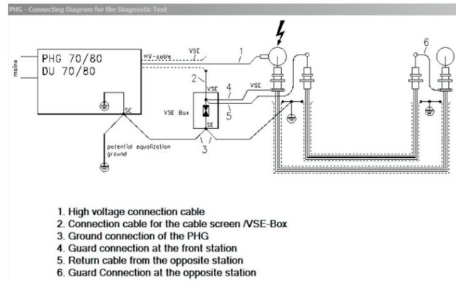
➤ Figure 51: Programmable high-voltage generator (PHG) connection diagram for TD with guard ring application
