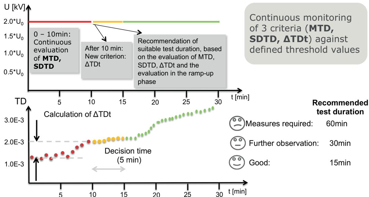
Figure 7: Illustration of MWT hold stage
