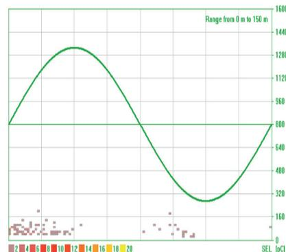
➤ Figure 87: PRPD pattern of cable section around 37 m, inner PD
