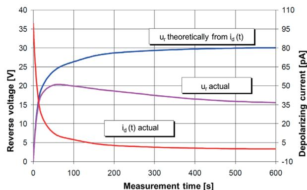
Figure 136: (Fig. 6 of [34]) Comparison between the return voltage calculated from depolarisation current and the practically measured return voltage
