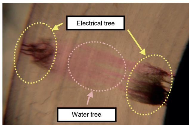
➤ Figure 28: Photo of actual water tree and electrical tree after dissection (XLPE cross section)
