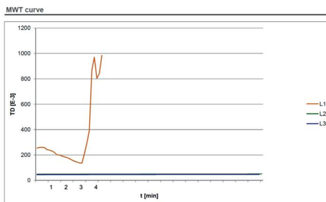
➤ Figure 13: Ref. 3730-31, MWT hold phase, joint breakdown after 4 minutes
