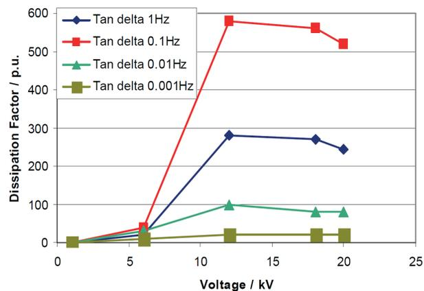
➤ Figure 23: Comparison of non-linearity in the frequency domain of a heavily water-tree-aged XLPE cable [Kus, 1998] [1]
