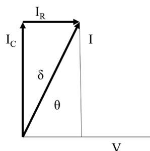
Figure 19: Extract from IEEE 400.2-2001, Fig. 6 – Phasor diagram for high loss dielectric material [13]
