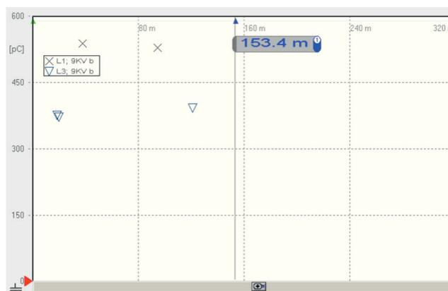
➤ Figure 116: PD on PILC cable after 10 min trending
