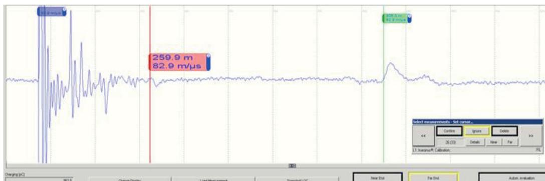
➤ Figure 77: TDR / calibration graph with identification of a joint with water ingress at 260 m
