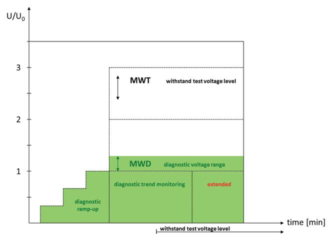
Figure 15: Monitored Withstand Diagnostics [15]
