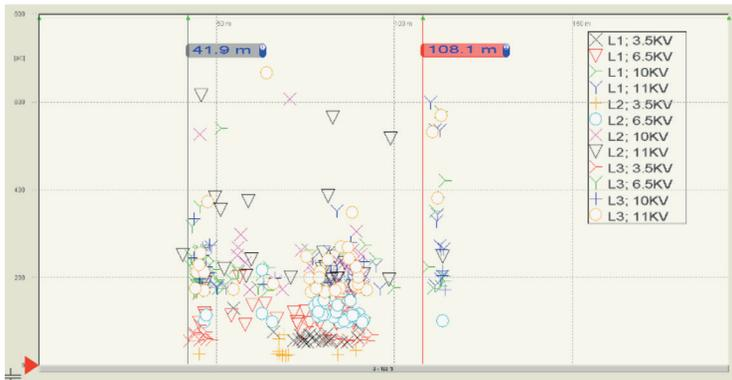
Figure 46: PD localisation graph – PILC cable with tracking in a joint, minor PD activities [20]
