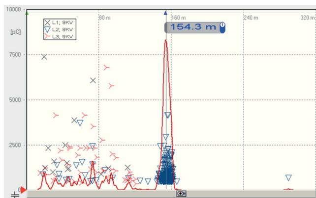
➤ Figure 115: PD on PILC cable, widely spread and PD cluster
