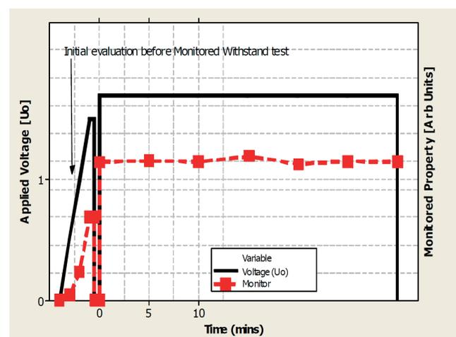
Figure 4: Schematic of a MWT (black) with optional diagnostic measurement (red) [14]
