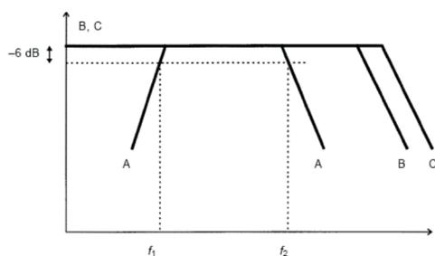
➤ Figure 64: Definition of measurement band width acc. to IEC 60270 [36]
