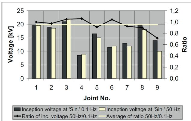
➤ Figure 82: Partial discharge inception voltage in comparison with HV source [24]
