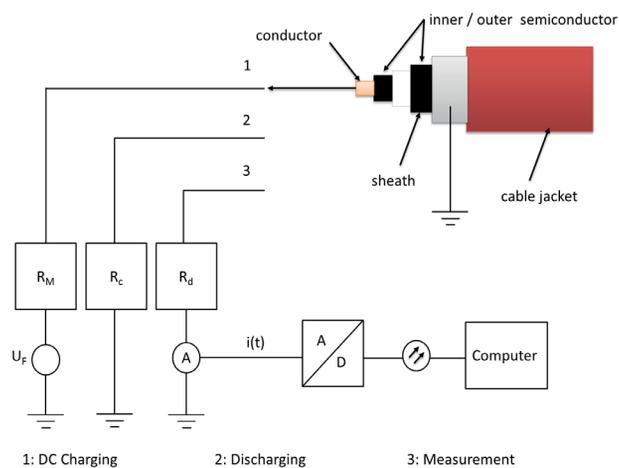
➤ Figure 131: Basic measurement circuit for the IRC analysis, KDA1
