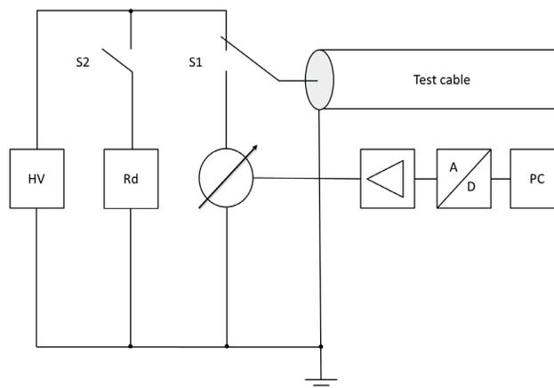
Figure 134: Block diagram of the return voltage method [16]
