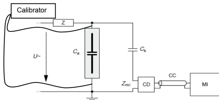
➤ Figure 65: PD measurement circuit acc. to IEC 60270 [36]
