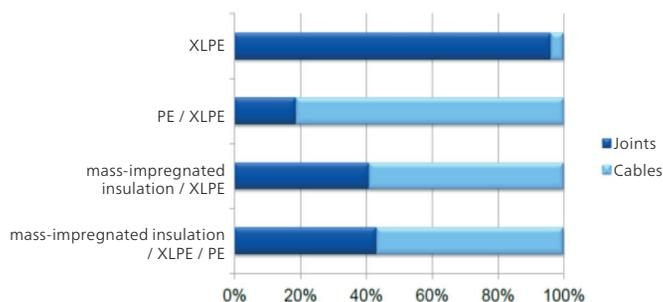
Figure 107: XLPE cables, mostly joint problems. Cable ageing in older cable systems. (Source: Mitnetz)
