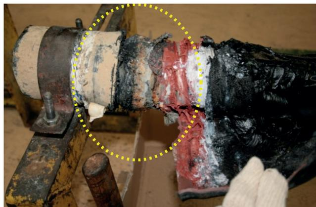
➤ Figure 148: Water found in cable during joint recovery. CAS corroded at Sumitomo cable side inside inner sleeve
