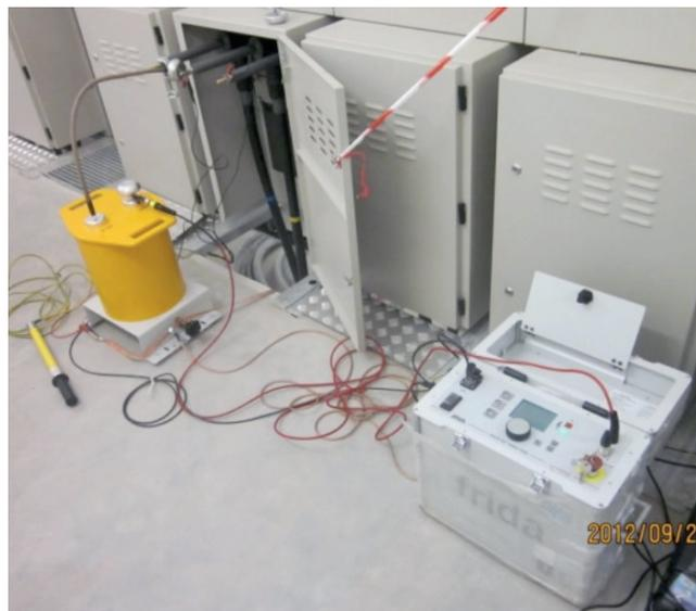
➤ Direct connection of light-weight PD TaD62 on the tower, close to the termination
