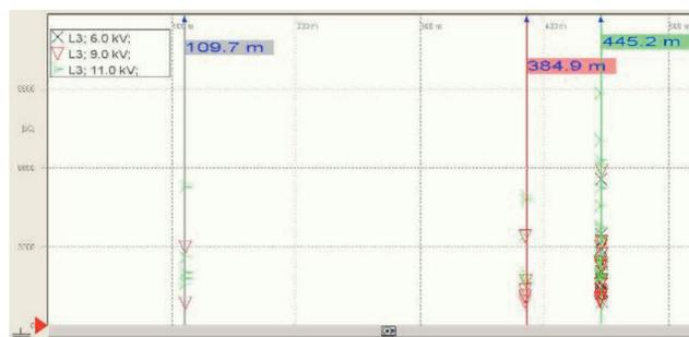
➤ Figure 63: PD localisation graph of a XLPE cable with 3 joints with PD activity
