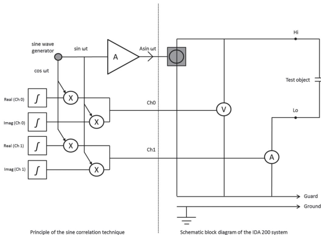
➤ Figure 137: (Fig. 10 of [23]) Schematic block diagram of the IDA 200 system
