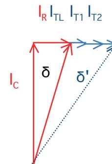
➤ Figure 53: Phasor diagram for visualising the influence of test lead and termination surface leakage current
