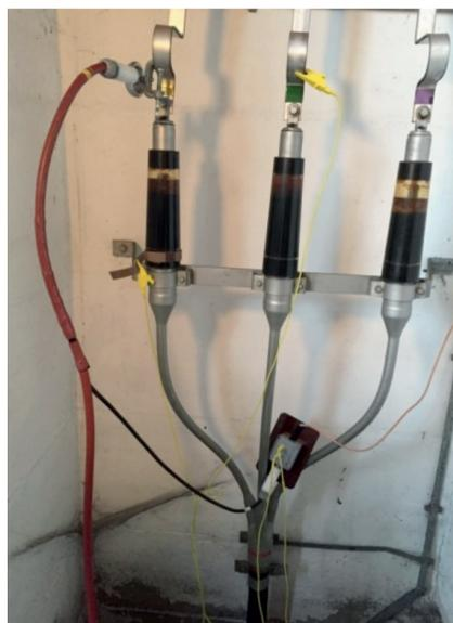
➤ Figure 54: TD measurement on open termination, PILC, oil filled termination, with and without VSE box – guard ring application, incl. busbar
