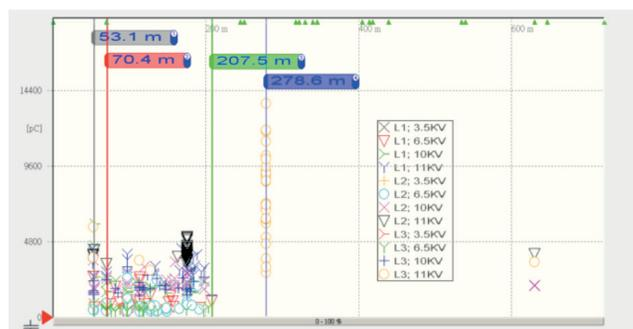
➤ Figure 69: Typical example of scattered PD activity along a PILC section (Ref. 11225)
