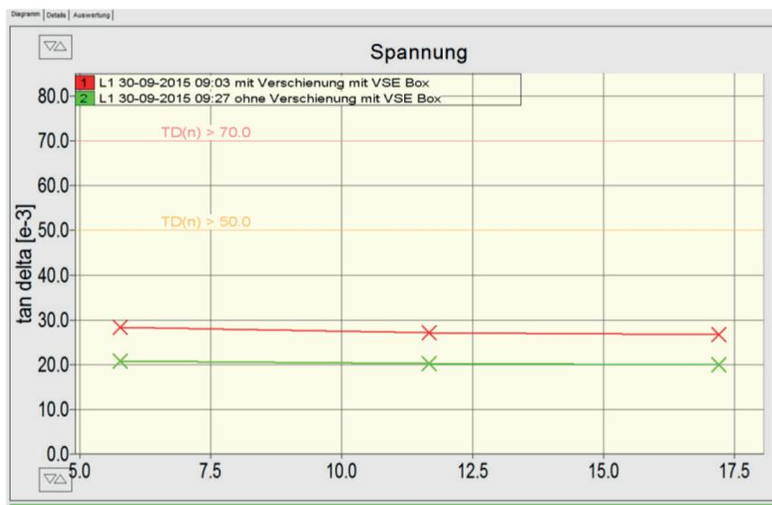
➤ Figure 57: TD result: 1. Including connected busbar, 2. With disconnected busbar
