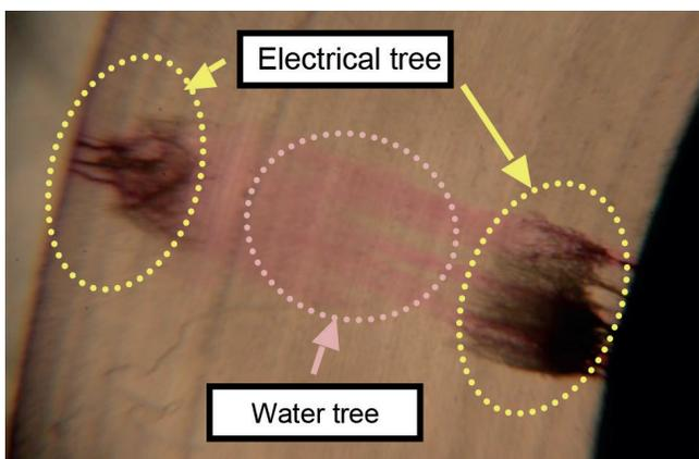
➤ Figure 151: Photo of actual water tree and electrical tree after dissection (XLPE cross section)
