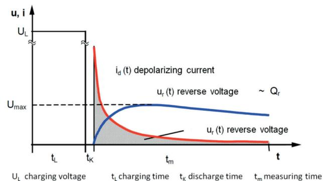
➤ Figure 132: (Fig. 5 of [34]) The principle of selected time-range based diagnostic methods
