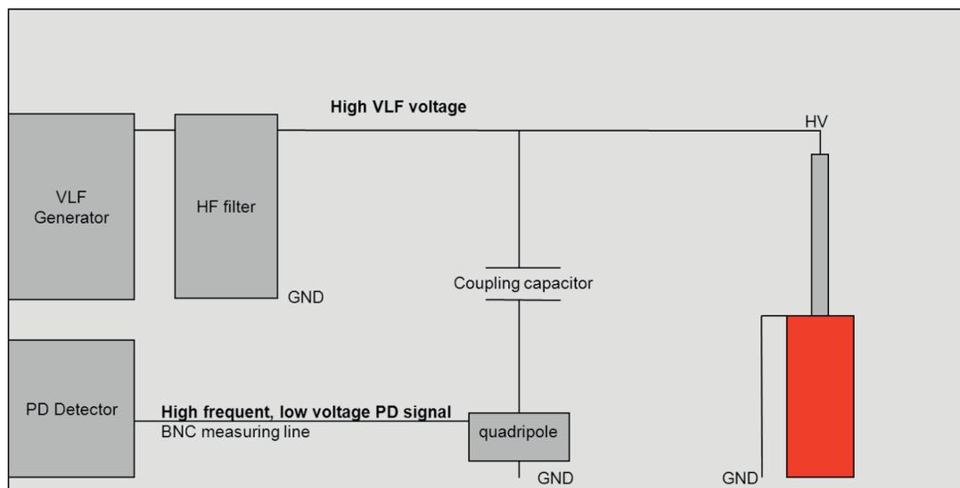
➤ Figure 66: Test setup of BAUR VLF PD system
