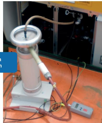
➤ Figure 72: CU60 PD coupler with calibrator
