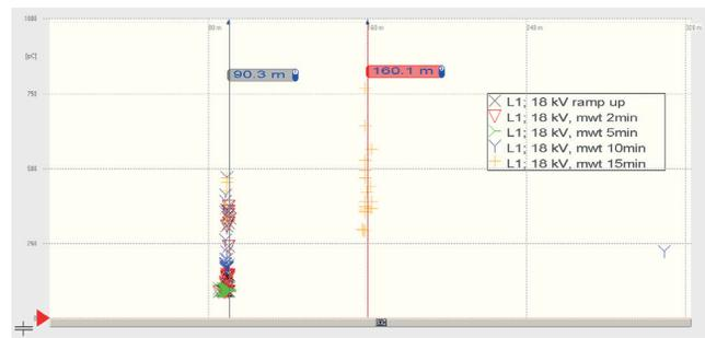
➤ Figure 16: MWT TD curve indicating the drying effect, MWT PD indicating PD over time
