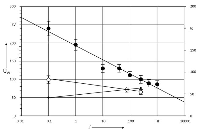
➤ Figure 1: Withstand voltage as a function of the frequency for model cables without and with mechanical damage [Goc, 2000]: [2]
