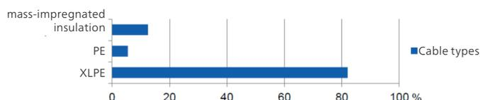
Figure 103: Total 16,000 km of MV cable (Source: Mitnetz)
