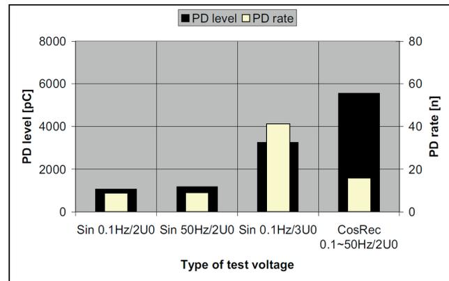
➤ Figure 83: PD levels with 0.1 Hz sinusoidal wave shape, 50 Hz power frequency and Cos-Rectangular 0.1 Hz [24]
