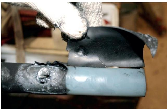
➤ Figure 149: Signs of water noted in insulation screen
