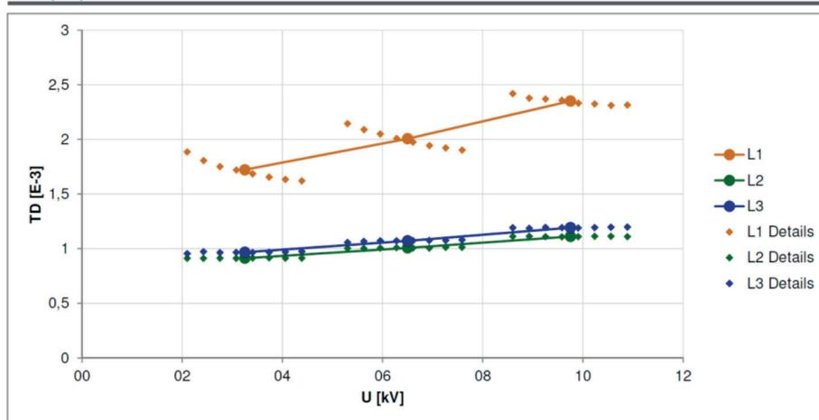
Figure 48: Ref. 2215CM, example L2, L3 stable condition, L1 water ingress in a joint
