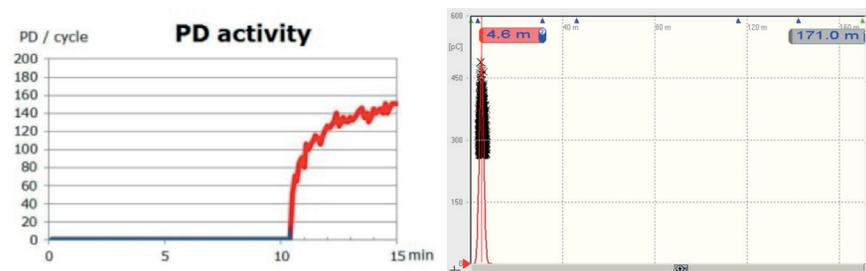
Figure 120: PD trending L2, PD cluster L2, at 4.6 m joint
