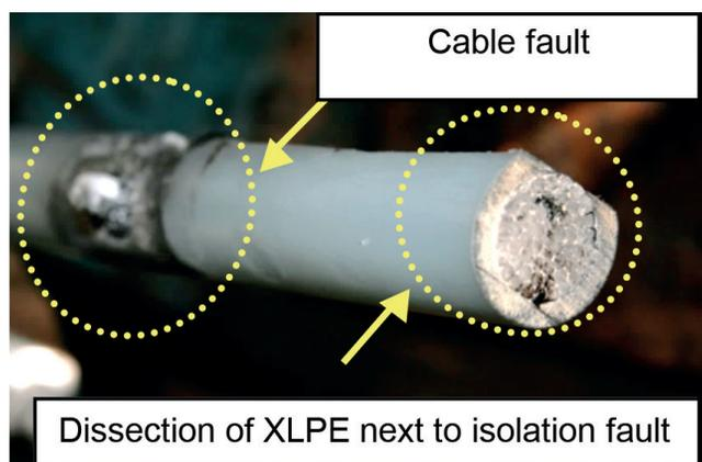
➤ Figure 88: Cable dissection of area close to cable fault
