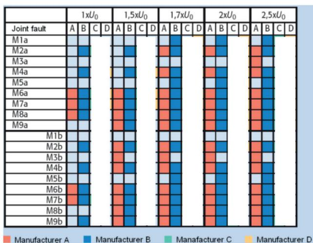
Figure 91: Test result matrix of VLF 0.1 Hz PD vs. 50 Hz PD, very comparable PD recognition ability
