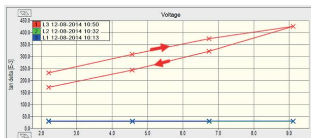
➤ Figure 60: VLF tan delta hysteresis measurement on a PILC cable
