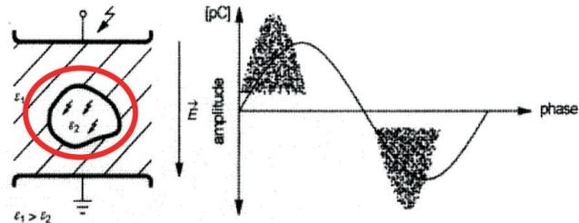
➤ Figure 110: PRPD pattern matching with reference void pattern; non-conducting material without direct contact with the metal electrode
