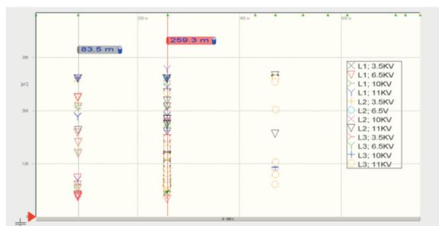
➤ Figure 70: Typical example of multiple joints showing PD activity (Ref. 6467)
