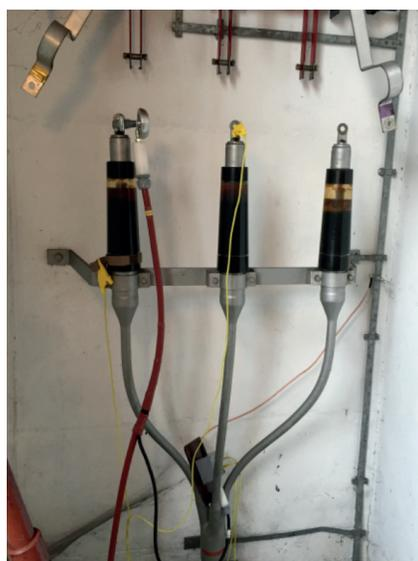
➤ Figure 56: TD measurement on open termination, connection with guard ring application, corona hood, disconnected busbar
