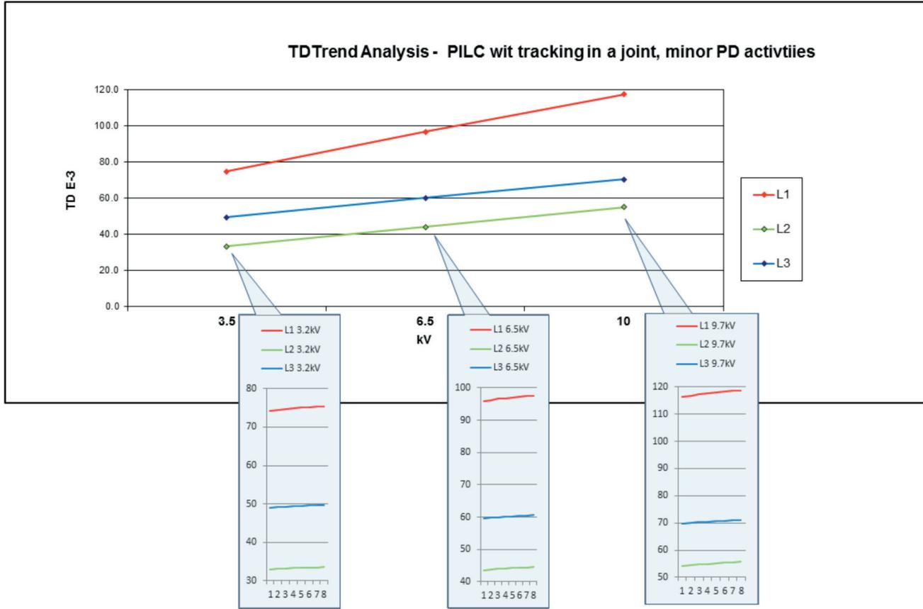
Figure 45: TD trend pattern – PILC cable with tracking in a joint, minor PD activities [20]
