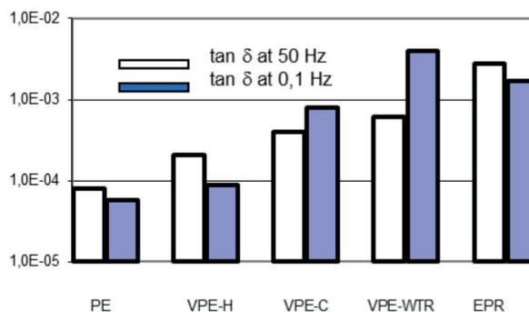
➤ Figure 20: Dissipation factor for new polymer insulated MV cables at 0.1 Hz / 50 Hz, (H: Homopolymer, C: Copolymer, WTR: Water Tree Retardant) [Kus, 1995] Fig. 4 [1]
