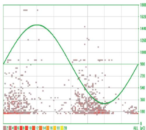
➔ Figure 81: Example for VLF 0.1 Hz, PRPD pattern, inner PD
