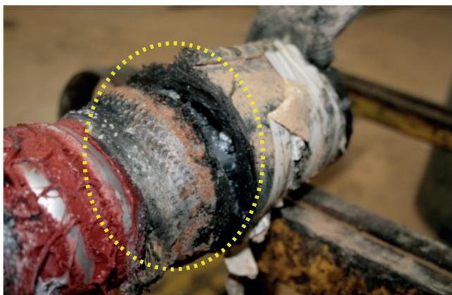
➤ Figure 147: Fault point on L3 at Sumitomo cable side near solder
