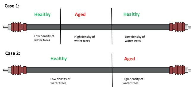
➔ Figure 32: Cable section with non-uniform water tree degradation
