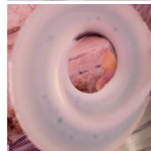
➤ Figure 30: Aged XLPE insulation, voids in XLPE, visible without colouring, 115 kV cable
