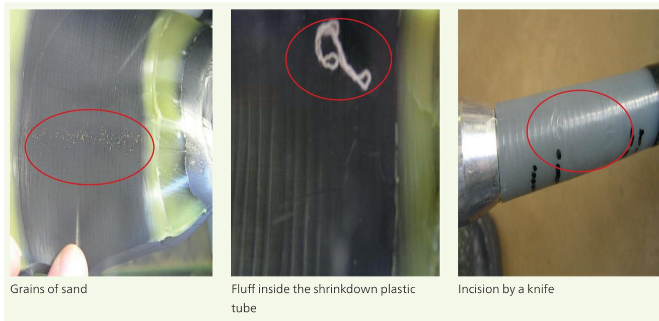
➤ Table 18: Examples of joint mounting faults
