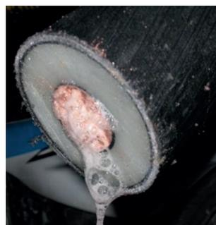
➤ Figure 29: Incomplete degassing of the cable in the factory after 14 months in operation
