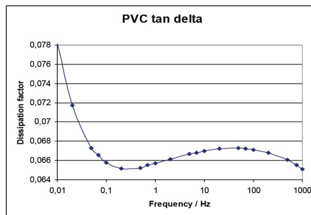
➤ Figure 21: Frequency domain spectroscopy of service-aged PE and PVC cables [1]
