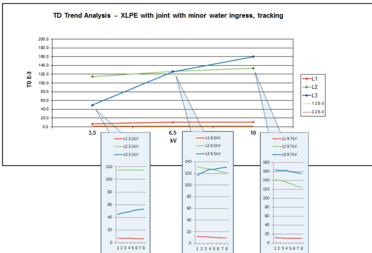
Figure 41: TD trend pattern – XLPE with joint with minor water ingress, tracking [20]
