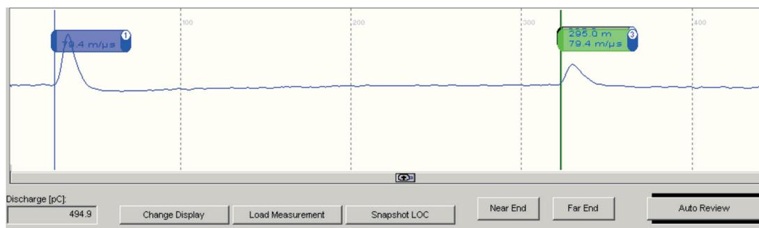
➤ Figure 74: TDR / calibration graph of a cable with 295 m without any joint
