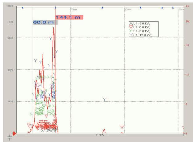
Figure 95: PD graph of mixed cable with scattered PD activity in PILC section
