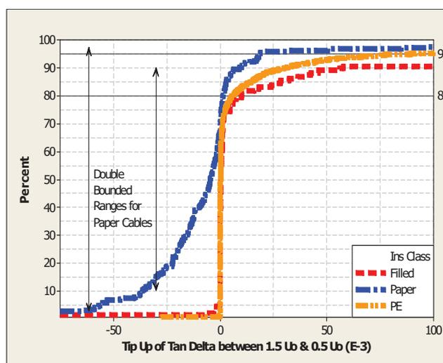
➤ Figure 58: TD tip-up distribution in filled, PILC and PE cables [22]
