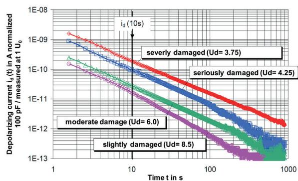
Depolarisation current normalised on 100 pF for differently water-tree-aged PE/XLPE homopolymeric cables.
