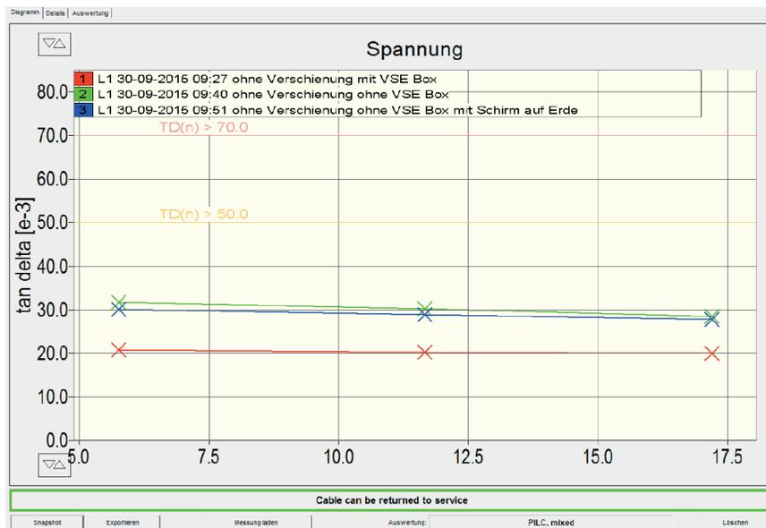
➤ Figure 55: TD result: 1. Connection with guard ring application, 2. Without guard ring application, 3. Without guard ring application, cable sheath additionally earthed => influence of surface leakage current visible
