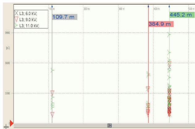
Figure 94: PD graph of XLPE cable with PD activity concentrated at 3 joints
