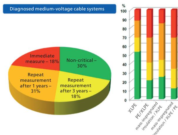
Figure 104: The result of cable diagnostics shows that pure XLPE cable circuits seldom require immediate action. With old types of PE cables and PE mixed with PILC cables, the diagnostics often reveal hidden and critical defects that have to be repaired within a few weeks or month. (Source: Mitnetz)
