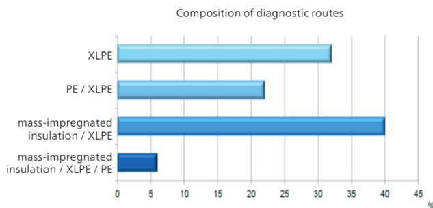
Figure 105: The selection of cables to be diagnosed; focus is placed on mixed cable circuits that are more prone to cable failures. (Source: Mitnetz)
