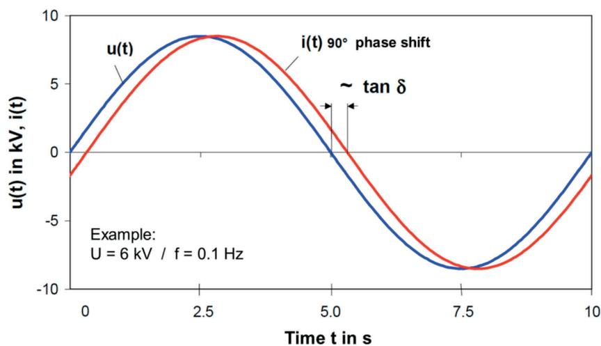
Figure 139: Tan delta measurement illustration [16]
