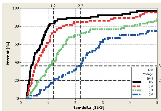
➤ Figure 31: Cumulative distribution functions of tan delta field data for > 10,360 m of cable measured [18]
