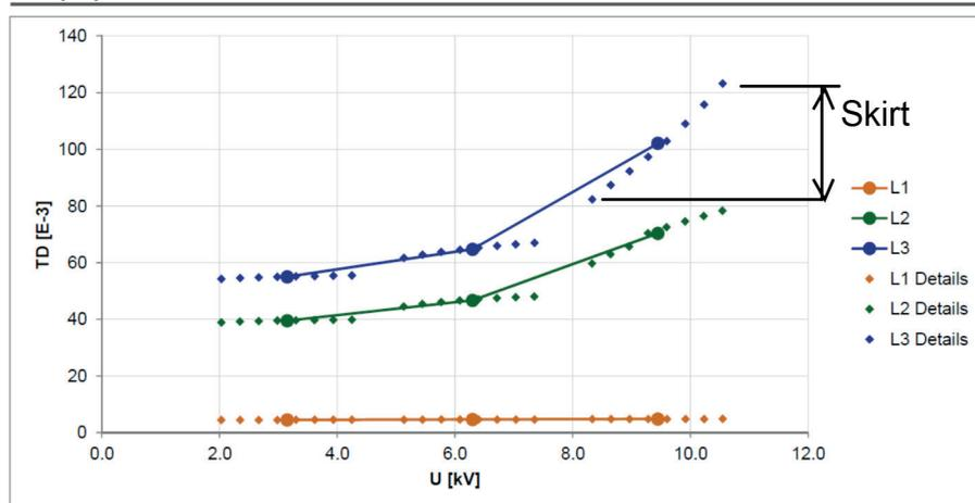
Figure 49: Ref. 8444CM, example L2, L3 tracking in joint, L1 stable condition
