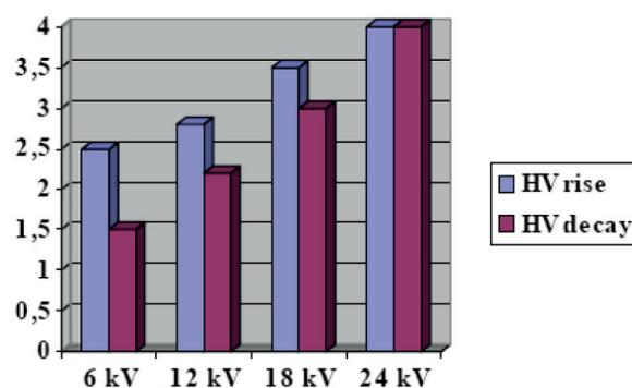
➤ Figure 59: Hysteresis of dissipation factor TD at VLF voltage rise and voltage decay [6]
