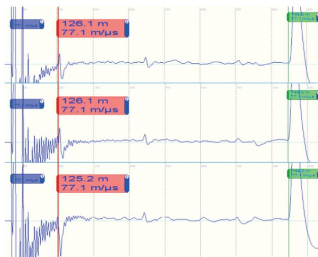
➤ Figure 113: TDR waveforms are inconsistent in polarity for three phases, Figure 2 of [29]
