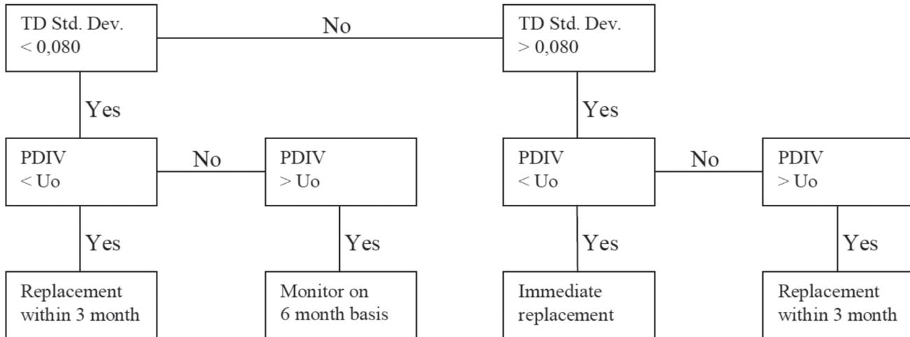
Figure 101: Joint PD categorisation logic > 2,000 pC
