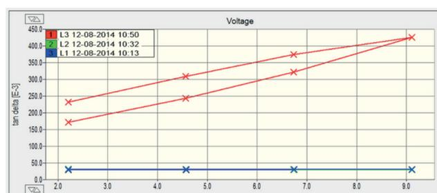
Figure 114: VLF tan delta hysteresis measurement on PILC cable
