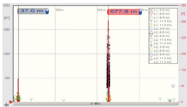
➤ Figure 86: PD localisation graph, suspicious PD activity at 37 m. Immediate breakdown during VLF test 2.
