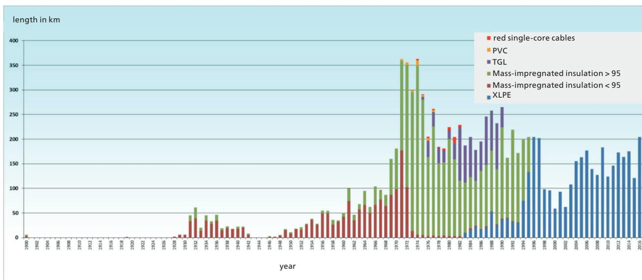
Figure 109: Type and ageing structure of 6/10 kV cables in Stromnetz Berlin GmbH, date 31.12.2016
