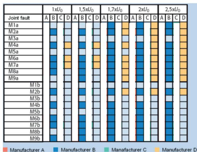
Figure 92: Test result matrix of 50 Hz PD vs. DAC PD, very inconsistent PD measurement ability by DAC
