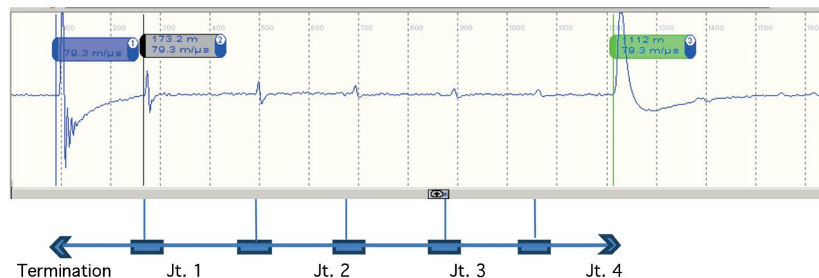
➤ Figure 75: TDR / calibration graph of a new XLPE cable with 6 equal sections and 5 joints
