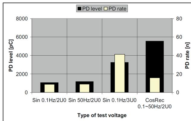
Figure 96: PD level and PD rate at selected types of test voltage [24]
