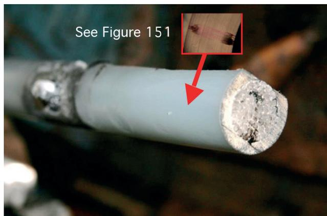
➤ Figure 150: Suspected water tree developed near to fault point
