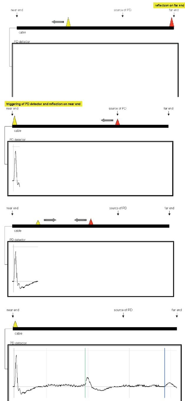
Figure 68: Sequence of graphical PD pulse localisation
