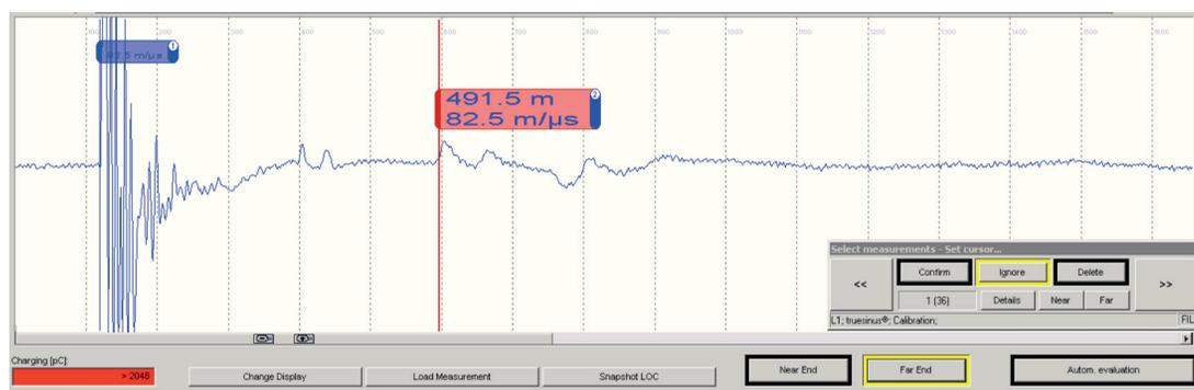
➤ Figure 76: TDR / calibration graph with identification of several joints, e.g. 491.5 m
