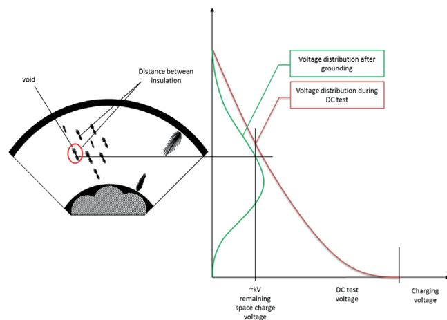
Figure 2: Space Charges in voids of XLPE during DC testing [5]
