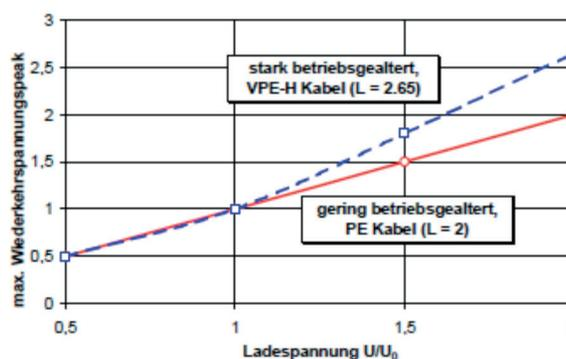
Peak of return voltage in relation to the charging voltage for differently aged PE/XLPE. (measurement example,  $t_L = 5$  min,  $t_K = 2$  sec.)
