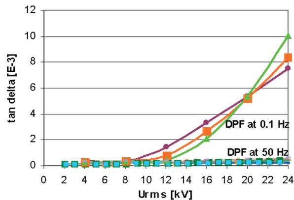
➤ Figure 22: Nonlinearity of DPF on service-aged XLPE cables at 0.1 Hz and at 50 Hz excavated and extracted in 2008 [1]
